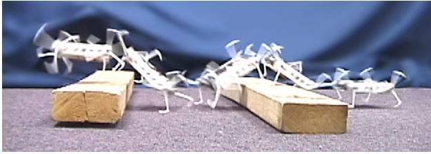
Figure 4. Composite of video frames showing Mini-Whegs IV traversing two 3.8cm high by 8.9 cm wide obstacles while running at 3 body lengths per second.
