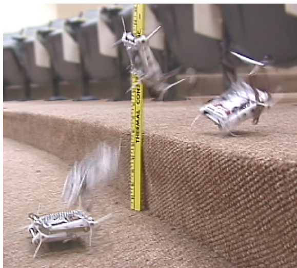
Figure 5. Composite of video frames showing Jumping Mini-Whegs clearing a 15cm high stair.
