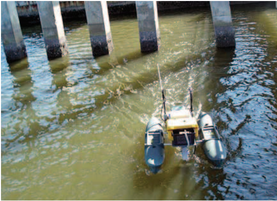
Fig. 50.4 Unmanned surface vehicle exploring the bridge to Marco Island, Florida (courtesy of CRASAR)
