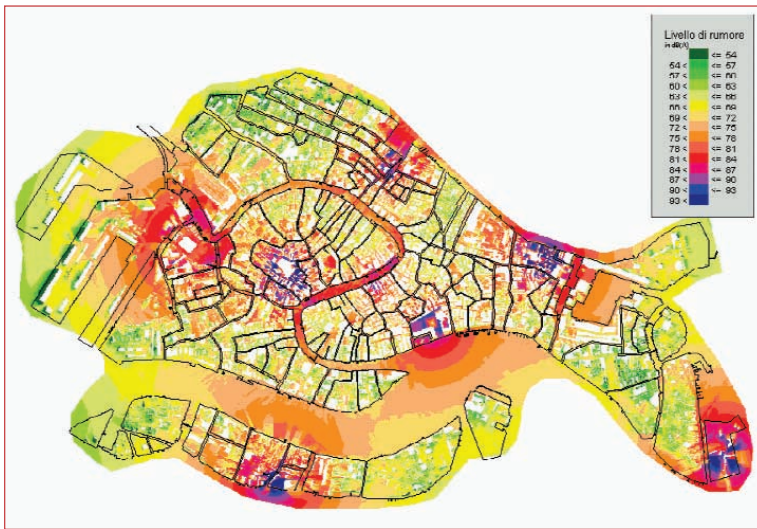
Figure 1. Noise map of alert system currently used in Venice. Colors represent sound-pressure level in dB(A). The sirens' coverage is far from uniform, and in many areas the sound levels are inadequate.
