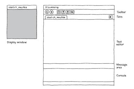
Figure 2-1. The Processing Development Environment.
