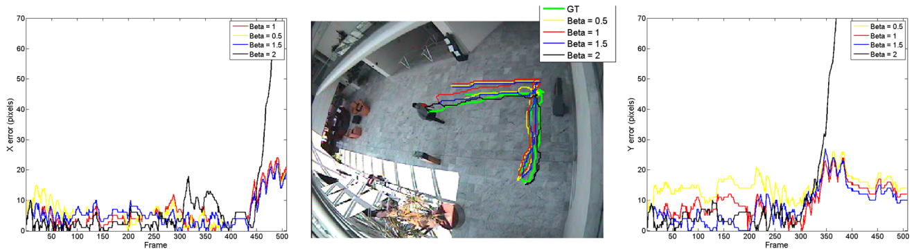
Figure 7: Centre image: Trajectories of the F-score tracker when varying \beta . Yellow: \beta = 0.5 , red: \beta = 1 , blue: \beta = 1.5 , black: \beta = 2 . Left image: error in pixels on the X coordinate compared with the ground truth. Right: error (in pixels) on the Y coordinate.
