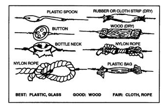
Fig. 4: Field-expedient insulators as suggested by the Sniper Training Manual [17].
