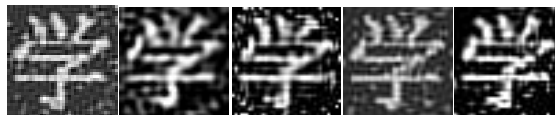
Fig. 14. Image reconstruction with M = 35 for 5% salt-and-pepper noise-contaminated binary image. From left to right are DCT and Legendre, Tchebichef, Krawtchouk ( p_1 = p_2 = 0.5 ), and Racah moments ( a = \alpha = 10 , b = 50 , and \beta = 5 ), respectively.
