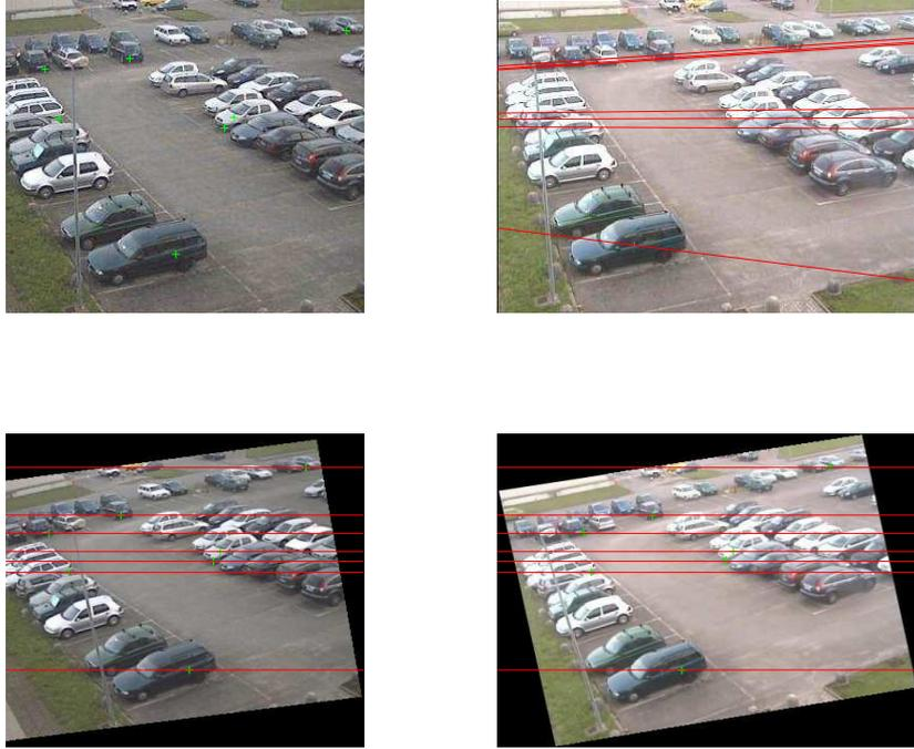
Fig. 7. Rectification of pair of stereo images having focal ratio 1.0. First row: pair of stereo images, Second row: rectified pair of stereo images.
