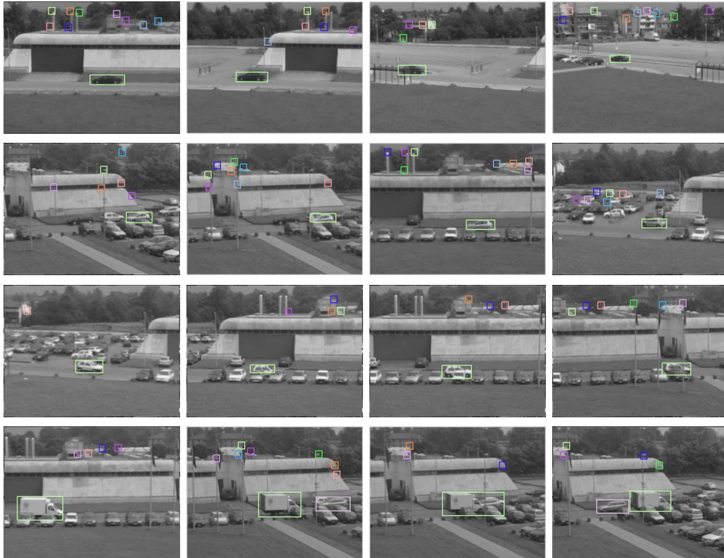
Fig. 8. Frames of test sequences with different zoom levels. The last three rows are characterized by a lot of objects that occlude the moving objects. The last row, in particular, shows a representative frame of a sequence where two vehicles cross their trajectories.
