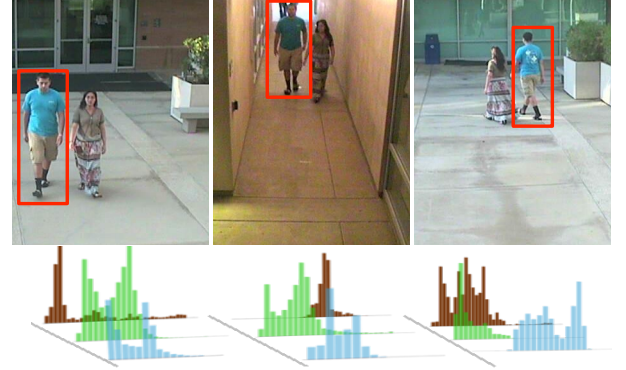
Fig. 1. Three images of the same person in three non-overlapping cameras from the RAiD dataset [1]. Below each image, HSV features are shown as 3 different histograms. Brown denotes the hue, green denotes saturation and the sky-blue denotes the value histograms respectively. The inconsistency of the histogram shape does not allow them to be used as unique features for re-identification.
