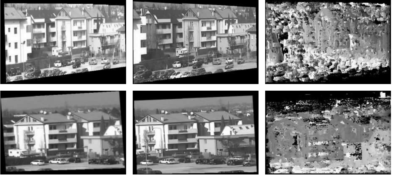
Fig. 14. Experiment for high resolution depth estimation in two successive iterations (top to bottom). In each row left camera image, right camera image and corresponding depth map image.
