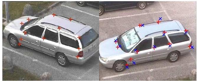
Fig. 7. SIFT ‘x’ and Chain of Homographies ‘+’ based correspondence between wide baseline stereo images.
