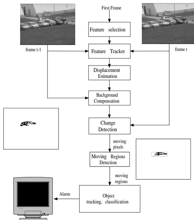
Figure 1: General architecture of the surveillance system
