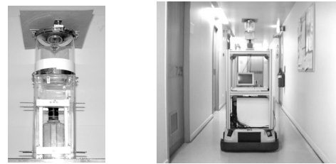
Fig. 2. Left: omni-directional camera. Right: camera mounted on the mobile robot.
