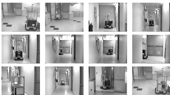
Fig. 15. A sequence of images of an experiment combining visual path following for door traversal and topological navigation for corridor following.
