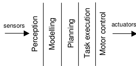
Figure 2.1: Phases of a deliberative control architecture.
