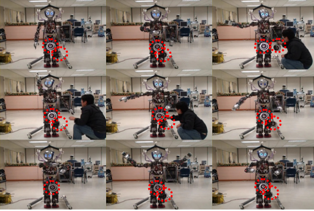
Fig. 19 Snap shots on balancing test of humanoid robot under unknown disturbances, Dotted circles indicate the dumbbells employed as unknown disturbances
