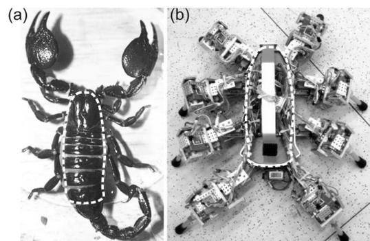
**Fig.5:** (a) The scorpion *Pandinus cavimanus* (Copyright 1996 by R. David Gaban [37] and reproduced with permission). (b) The eight-legged walking robot AMOS-WD08. Dashed lines show a body contour.
