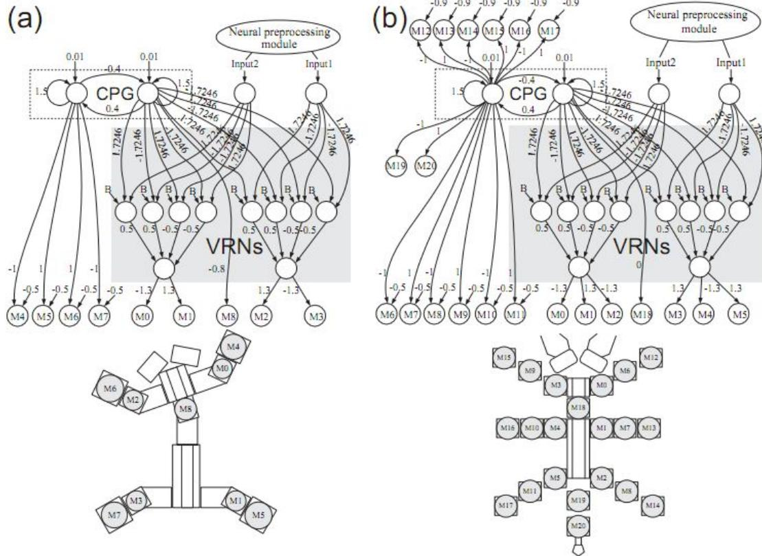
**Fig.8:** (a) Modular neural locomotion control of the four- (AMOS-WD04) and six- (AMOS-WD06) legged walking robots (Figs 3(b) and 4(b)). It consists of two modules: CPG and VRNs. All connection strengths and bias terms are indicated by the small numbers except the bias terms of the VRN given by  $B = -2.48285$ . The location of motor neurons  $M_i$  on the walking robots is depicted below. We refer the reader to [31, 32] for more details of the controllers.
