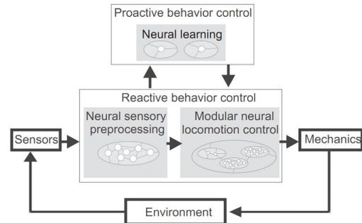
**Fig. 6:** Diagram of neural mechanisms of the walking robots. The sensor signals are passed through the neural preprocessing unit into the modular neural locomotion control unit which directly drives the actuators. In addition, the neural learning acts as high level control. It is used for enabling the robots to adapt to different situations. This neural learning mechanism leads to the generation of the proactive behaviors.
