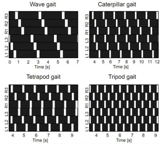
**Fig.13:** Examples of four different gaits observed from the motor signals of the CTr-joints. Black areas indicate ground contact or stance phase and white areas refer to no ground contact during swing phase. These gaits are similar to those found in insects [43].
