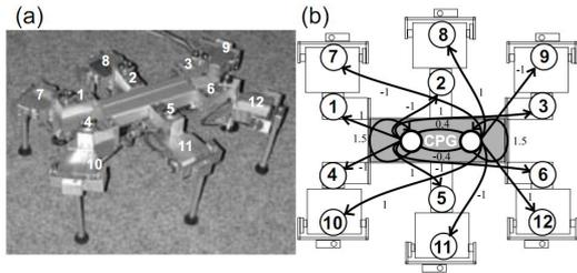
**Fig. 7:** (a) The physical six-legged walking robot *Morpheus*; each leg has two DOF. (b) The evolved neural control with only two hidden neurons (shaded area) and symmetric output weights to motor neurons (small black numbers). It performs as a quasi-periodic oscillator or a CPG, enabling an efficient forwards movement [39]. Note that the large circled numbers indicate motor neurons (corresponding to the numbered location of actuators in (a)).
