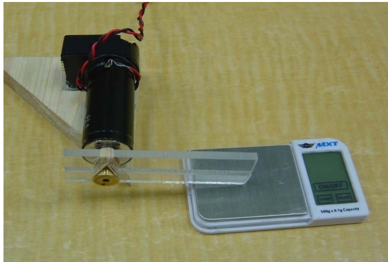
Figure F- 1: Test setup for Maxon motor calibration.
