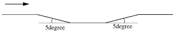
Figure 7 Test terrain with downhill, flat, and uphill components. This terrain was used to test the adaptability of the evolved neural controllers for the biped. Note that the robot has never experienced this environmental configuration during its evolutionary processes.
