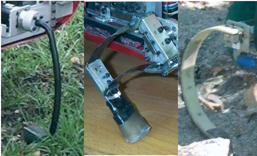
Fig. 5. Three generations of RHex legs. RHex's legs are designed to afford three degrees of passively compliant freedom so arranged that the radial 'spoke' direction is much more compliant than the relatively stiff lateral and tangential bending axes (Moore and Buehler, 2001). While the initial homogeneous (Delrin, left panel) legs and early succeeding generations of passively sprung four-bar (middle panel) leg constructions enforced point contact between toe and ground, the most successful designs are formed in 'half-circle' configurations (right panel) that promote a complicated rolling contact with the ground (Moore and Buehler, 2001).
