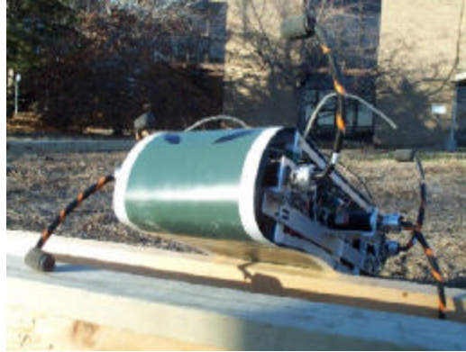
Figure 5: RHex [28] is a typical example of a Type 3 robot. Each leg is a single compliant spoke, driven, at the hip, by a motor under PD control. The spoke swings in a full circle parallel to the sagittal plane of the robot. RHex is a simple and reliable hexapod robot with good rough terrain capabilities.
