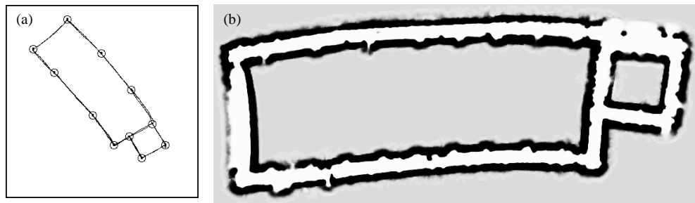
Figure 6. (a) Maximum likelihood map, along with the estimated path of the robot. (b) Occupancy grid map constructed using these estimated locations.
