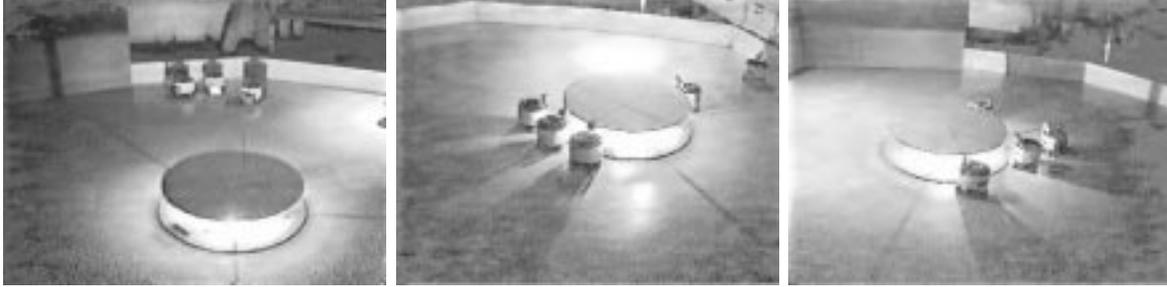
Fig. 8. Shown are five robots pushing a round box from its initial position first towards a goal-light in the right of the picture and then towards a goal-light on the left of the picture. The mpeg video from which this sequence was taken is available at <http://www.cs.ualberta.ca/~kube/>
