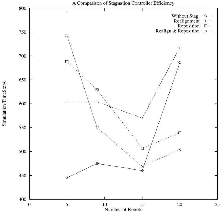
Fig. 4. The task efficiency results of four controllers with and without stagnation recovery behaviors. Shown are the average number of simulated timesteps taken to move the box 200 units from its initial position as a function of the number of robots. Reprinted with permission ©IEEE.
