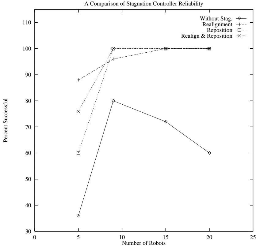
Fig. 3. The results comparing box-pushing controllers with and without stagnation recovery behaviors. Success was defined as pushing the box 200 units from an initial position within 2000 simulation timesteps. Each data point represents the average of 25 trials with percentage successful shown as a function of the number of robots. Reprinted with permission ©IEEE.
