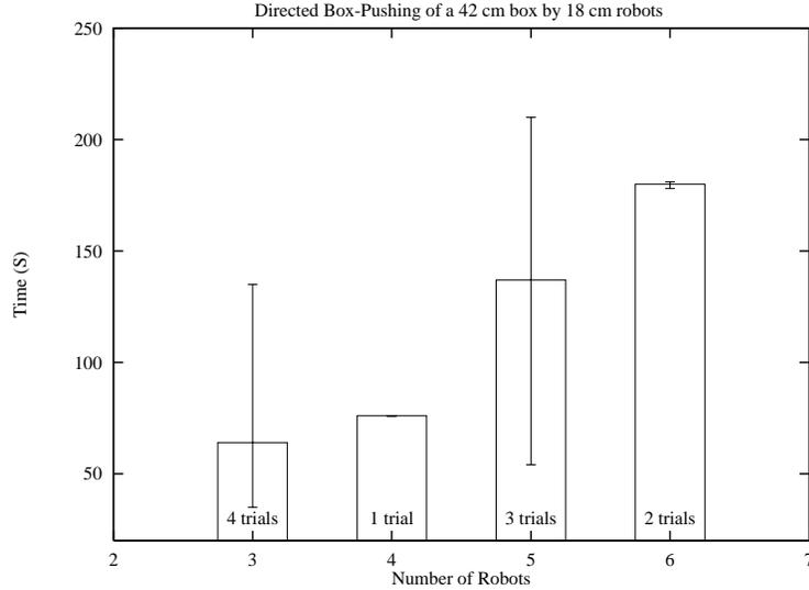
Fig. 9. The mean execution time of moving a  $42^2$  centimeter box 2.5 meters towards a goal position (P5, P6, P7) as a function of the number of robots. For each plot the number of trials as well as the minimum and maximum run times are indicated. A boxside is approximately twice the robot’s diameter and increasing the number of robots increases the robot interference as they compete for the limited space available.
