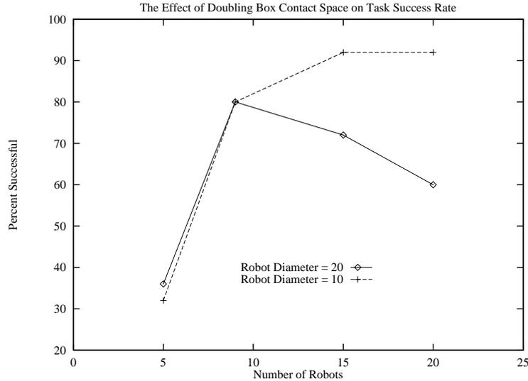
Fig. 10. The effects of doubling box contact space on the task success rate. The results from two simulation experiments in which the only parameter changed was the robot’s diameter, with the size of the box side fixed at 90 units. Robot diameters of 20 and 10 were compared for a task in which a box was moved 200 units from its initial position. Each data point is the average of 25 simulation runs each with a different random initial configuration.
