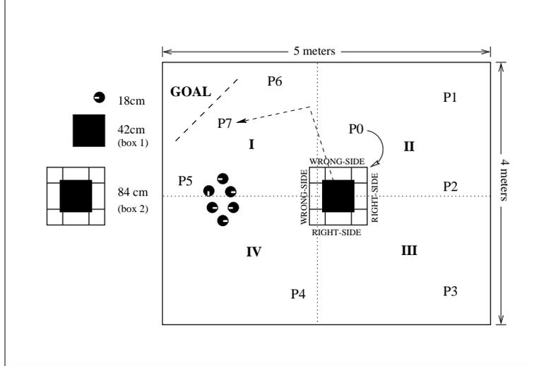
Fig. 5. In each trial the box was placed at initial position three meters from the goal line and the robots were placed at one of the indicated starting positions labelled  $P_1 - P_5$ . After Kube and Zhang [31]. Reprinted by permission ©Kluwer Academic Publishers.
