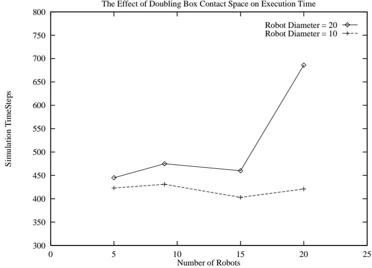
Fig. 11. The effects of doubling box contact space on execution time. The results from two simulation experiments showing execution time versus system size. The only parameter varied was the size of the robot; the size of the box side was held constant at 90 units.
