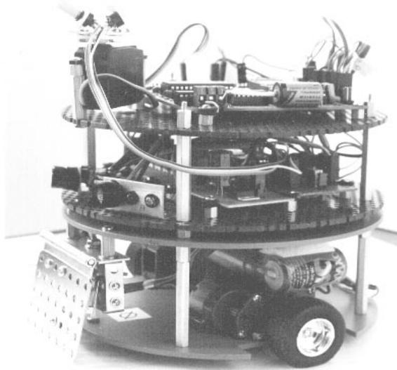
Fig. 6. Each of the robots are equipped with two forward pointing infrared obstacle sensors, one touch sensor, two CdS box-tracking photocells, and a destination sensor, all mounted on a differentially steered base.
