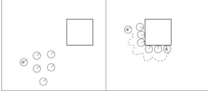
Fig. 2. A FOLLOW and GOAL behavior produce coordinated motion towards a box. While the AVOID behaviour causes robot “A” to disperse around the box until an empty spot is found.
