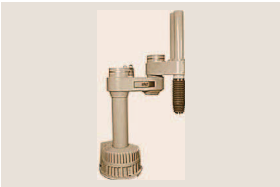
Fig. 3.14 The Adept robot uses closed-loop control and variable-reluctance motors
