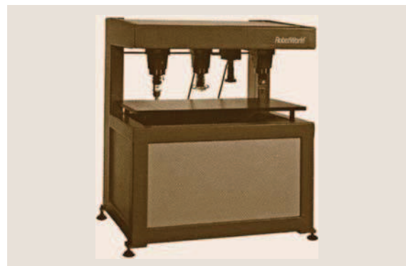
Fig. 3.12 RobotWorld is an integrated workcell with multiple robot modules that move on air bearings
