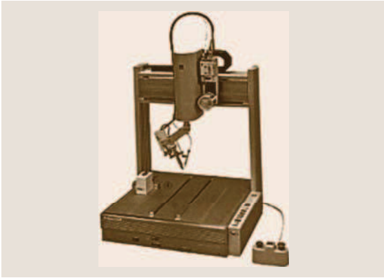
Fig. 3.13 The Sony robot uses open-loop permanent-magnet stepper motors
