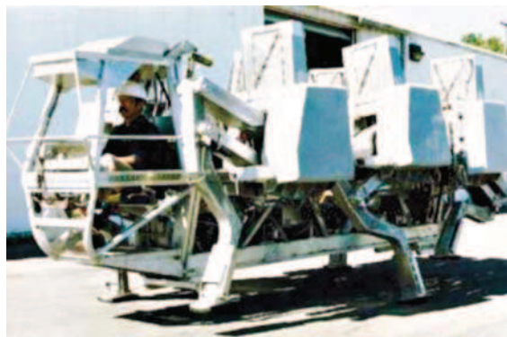
Fig. 16.30 The adaptive suspension vehicle (1986) [16.58]
