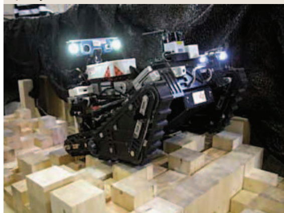
Fig. 48.20a,b Mobile platforms with passive adaptation: (a) Soleo-Shrimp [48.57] and (b) Robhaz-dt3
