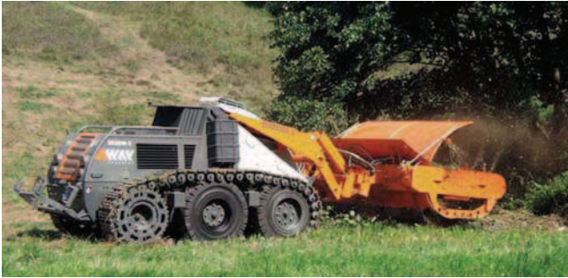
Fig. 48.7 Bozena teleoperated demining vehicle (Way Industry, Slovakia)
