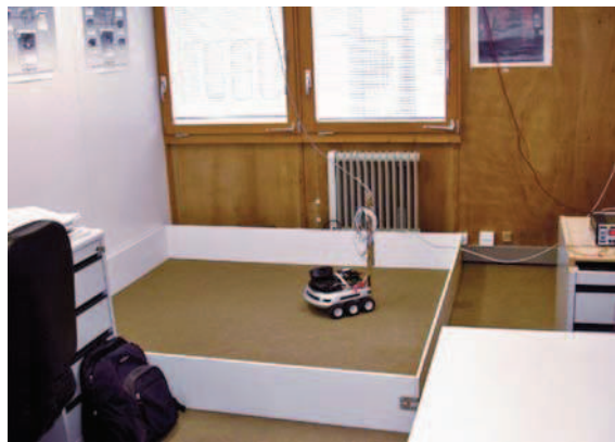
Fig. 61.14 A mobile robot with a pan-tilt camera is asked to move within the walled arena in the office environment
