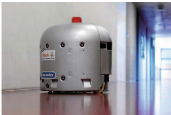
Fig. 54.23 Professional cleaning robot Robo40 navigating on smart floor
