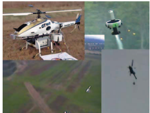
Fig. 44.15 Georgia Tech’s unmanned helicopter in a parent–child configuration. The child is a hover-capable ducted fan
