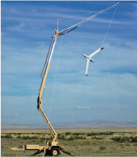
Fig. 44.13 Skyhook system in action (courtesy Insitu, Inc.)
