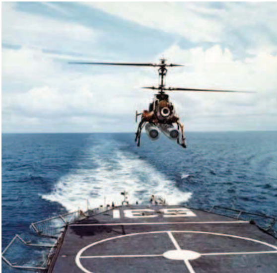
Fig. 44.2 QH-50 DASH unmanned helicopter on final approach (US Navy)
