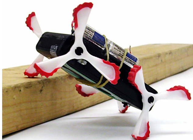
Fig. 2 Mini-Whegs™ 7 can climb obstacles 25% greater in size than the length of each leg spoke.
