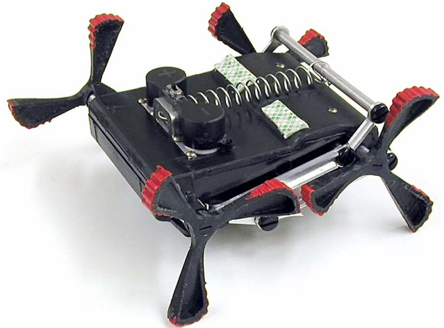
Fig. 1 Mini-Whlegs™ 9J, a 10.4 cm long robot that runs and jumps.
