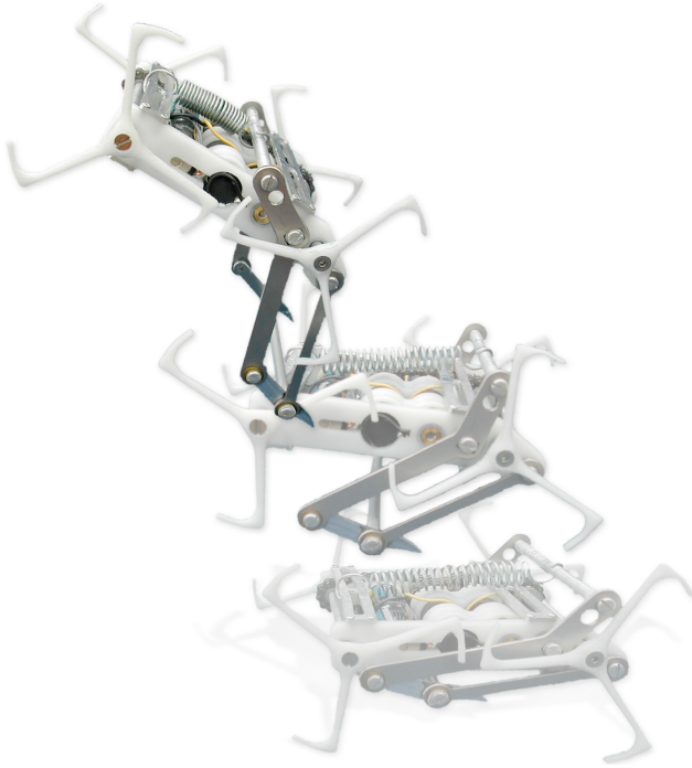
Figure 3. Photographs illustrating the parallel four-bar linkage used in Jumping Mini-Whegs.
