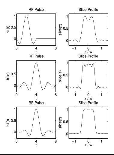
How applicable is the **small tip angle** assumption? Actually FT approach works well even up to  $90^{\circ}$  tips! So we can use Fourier methods (filter design) to choose  $b_1(t)$ .
