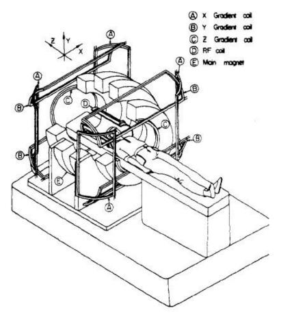
A typical superconducting magnet is based on niobium-titanium (NbTi) alloys, requiring a liquid helium cryogenic system that cools to about  $4.2^{\circ}$  K.
