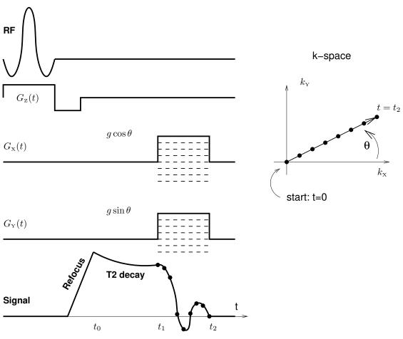
The above **pulse sequence** illustrates the sequence of excitation/readout phases. The sequence is repeated for many  $\theta$  values. For  $t \in [t_0, t_1]$ , there is (ideally) no change in the transverse magnetization (for z = 0) except for  $T_2$  decay, which we have ignored in deriving the signal equation. So the baseband signal (which is not sampled during this time but could be) is just the DC component of m(x, y), the transverse magnetization pattern established by the RF excitation.
