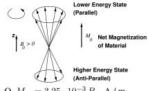
At 37° C = 310° K, for a single proton in H<sub>2</sub>O,  $M_{z0} = 3.25 \cdot 10^{-3} \, B_{z0}$  A / m.
