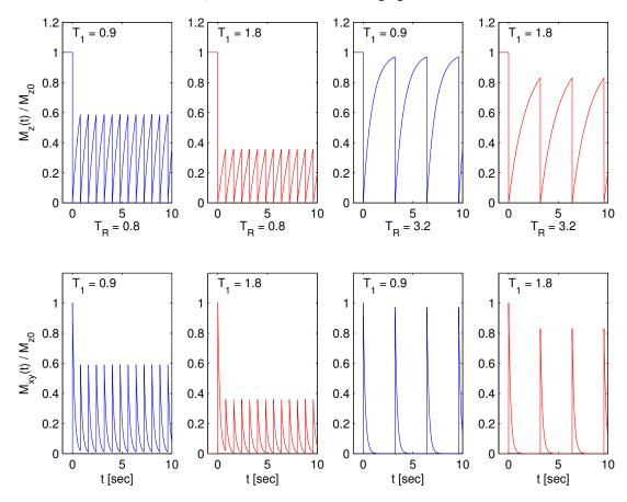
The kind of sequence illustrated above is called **saturation-recovery** imaging; it assumes the transverse component has decayed essentially to zero before the next excitation, which requires that  $T_R \gg T_2$ .
