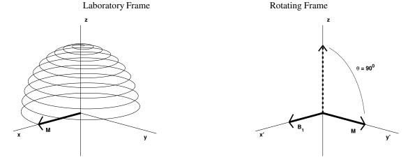
If the RF strength and duration is just right, then one can tip the magnetization into the transverse plane. (A 90° **flip angle**). Usually this type of excitation yields the largest signal (for a single excitation).
