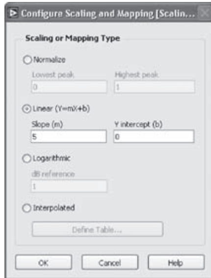
Figure 2-33: Configuration of Scaling and Mapping Express VI.
