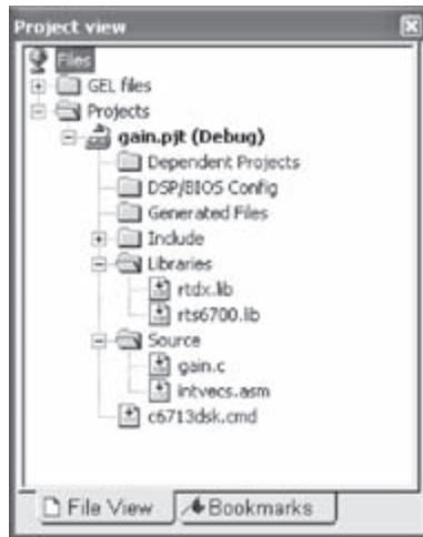
Figure 9-4: Project view of CCS.
