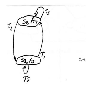
*U* is a strongly connected subgraph (no decomposition is needed)
