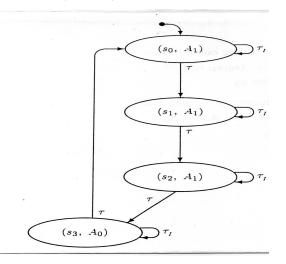
The subgraph  $S = \{(s_0, A_1), (s_1, A_1), (s_2, A_1), (s_3, A_0)\}$  is an **adequate subgraph**, as it is both fair ( $\tau$  is taken in *S*) and fulfilling ( $\Diamond(x = 3)$  belongs to both  $A_0$  and  $A_1$ , but x = 3 belongs to  $A_0$ )
