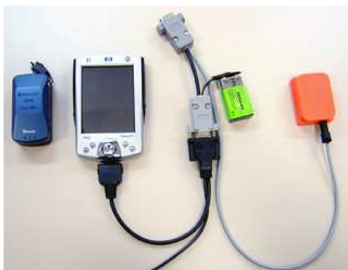
Figure 5. Prototype recognition platform. From left to right: Bluetooth enabled GPS, PDA, RS232 connection with battery, Orientation Sensor
