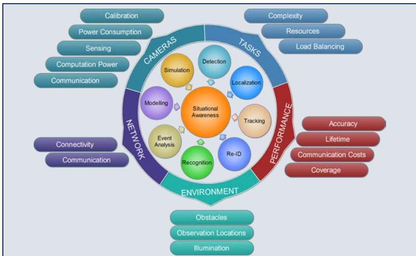
Figure 2 Self-reconfiguring smart camera networks deal with five elements: environment, cameras, tasks, network and performance. Considering all these elements, smart cameras cooperate network-wide to find a configuration that maximizes situational awareness, which is achieved through the distributed and parallel execution of tasks such as detection, tracking and event analysis.
