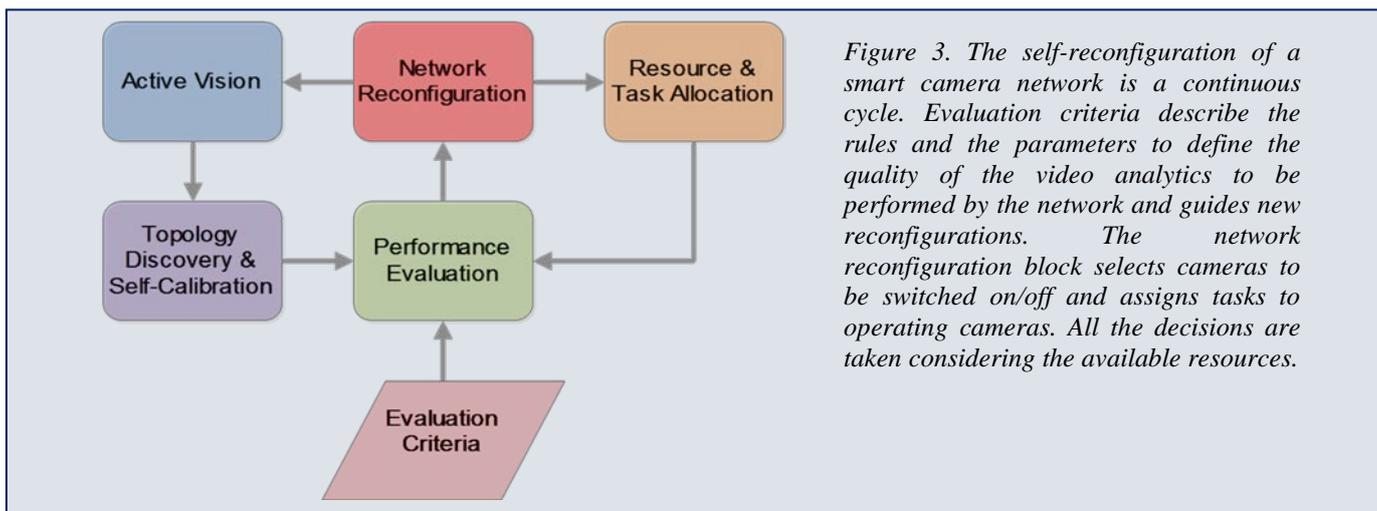
Figure 3. The self-reconfiguration of a smart camera network is a continuous cycle. Evaluation criteria describe the rules and the parameters to define the quality of the video analytics to be performed by the network and guides new reconfigurations. The network reconfiguration block selects cameras to be switched on/off and assigns tasks to operating cameras. All the decisions are taken considering the available resources.
