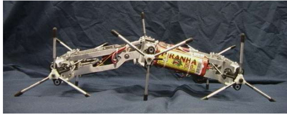
Figure 7. Whogs II can flex its body.
